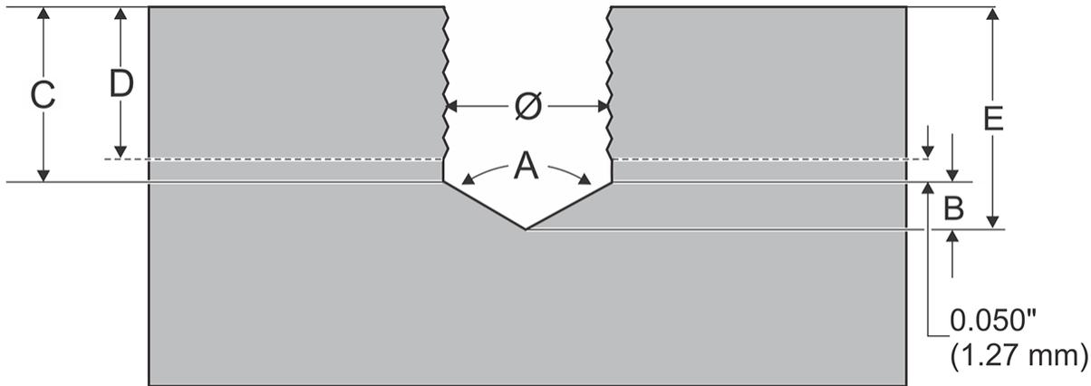
The full-diameter depth [C] of the hole is shallower than what is programmed because of the drill tip angle on the drill [A]. Program the full-diameter depth [C] at least 0.050" deeper than the tap depth [D].
