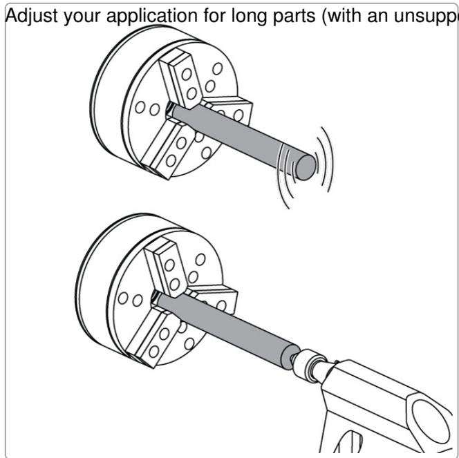
Adjust your application for long parts (with an unsupported length-to-width ratio of more than 3:1): Lower the cutting load through adjustments to the tool selection or program. Stiffen the workholding with supports, if possible. If your lathe has workpiece support equipment, such as a tailstock or a steady rest, be sure to use it.
