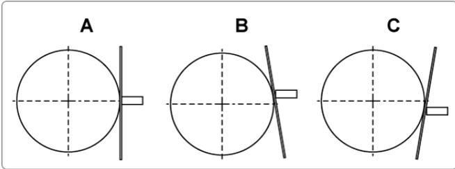
One way to check your tool's alignment with the spindle centerline:
