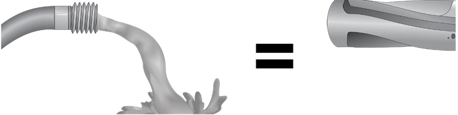
When there are a small number of coolant holes, or the coolant holes are small, less coolant is allowed to flow. But the restriction causes the coolant pressure to increase, and the coolant velocity increases. In this example, a tool with small coolant orifices is compared to a hose with a fitting on the end. The flow looks like this:
