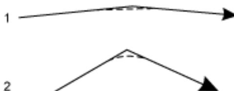
Use this setting to smooth out the motion of the machine in corners, or to make the machine more accurate when trying to hold a close tolerance.
