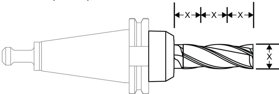
In some cases it may be necessary to use an extended tool, machining a deep pocket for instance. In these scenarios you must reduce the load on the tool by reducing the depth-of-cut, width-of-cut, RPM or feedrate to maintain a stable cut.
