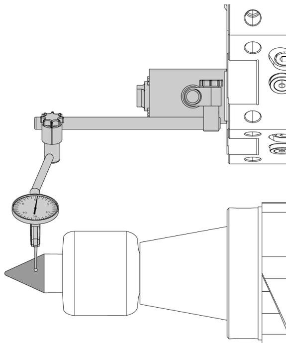
Check for bearing wear by gripping the point firmly and rotating it in one direction. The spindle should turn freely, if you can feel hesitations or roughness this indicates bearing wear.
