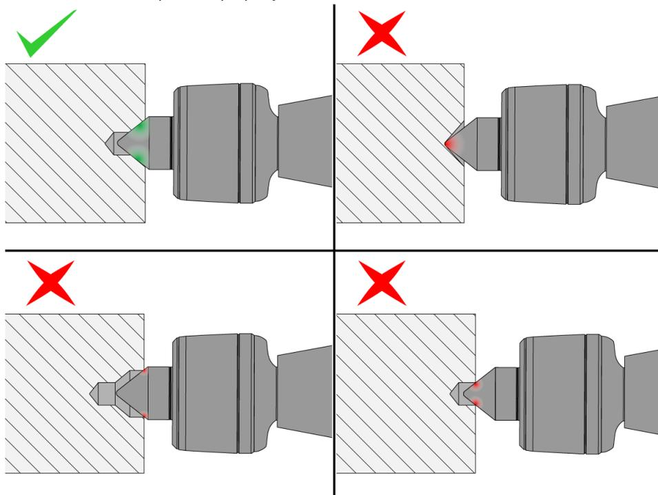
Be sure to use a 60° center drill tool. Countersink tools do not have the tip relief required for the live center.
